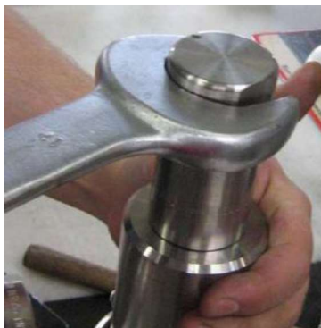
Fig. 1 Installing the cap
