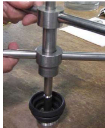
Fig. 7 Installation of the Elmoster bellows
