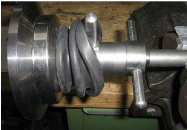
Fig. 7 Installation of the Elmoster bellows
