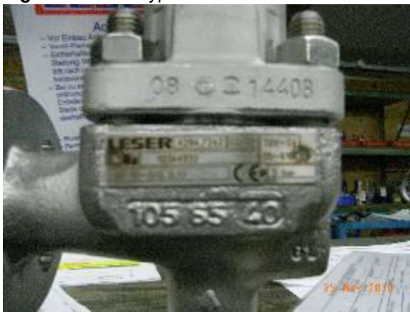
Figure 6.2.1-6: Standard plate on a flanged valve
