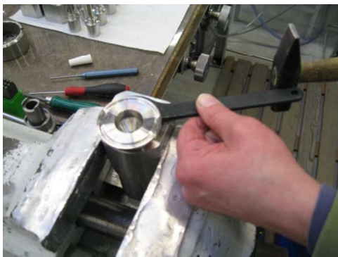
Fig. 5 Installation of the O-ring disc with a pin-type spanner wrench
