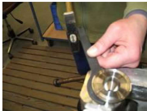
Fig. 6 Installation of the O-ring disc
