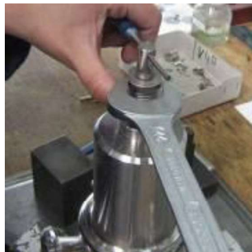
Fig. 2 Pressure setting of the safety valve
