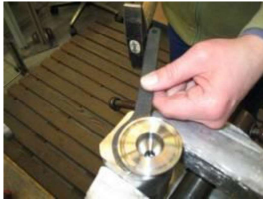
Fig. 4 Installation of the O-ring disc
