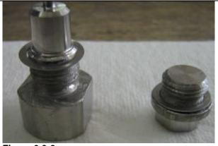
Grease a spacer ring for each of the screws and put on as a seal.
