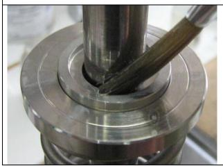
Put the bearing washer on the axial needle roller and grease.
