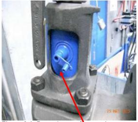
Figure 6-1: Protective cap for open bonnet
