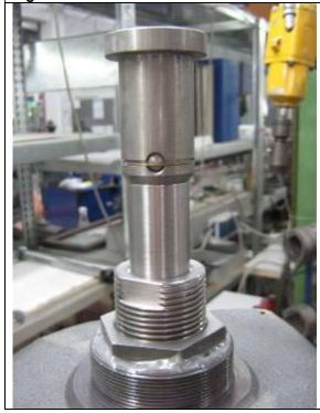
Remove the retaining clip and pin. Pull the spindle cap off the spindle.
