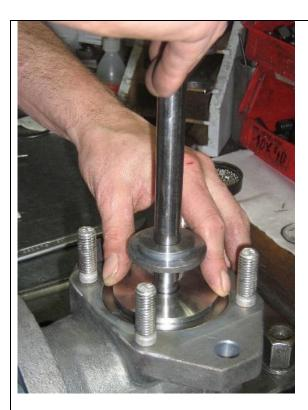
Insert disc-/spindle construction group carefully into the body.
