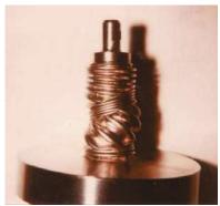
Figure 17.4-1: Twisted stainless steel bellows
