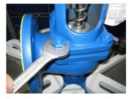
Fig. 1 Unscrewing a screw connection
