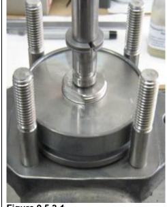
process, push the guide washer down and lift the spindle somewhat so that the disc does not touch down. Carefully put the disc with the
