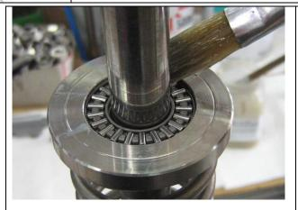
If applicable, grease the axial needle roller on the top spring plate.
