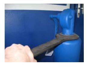
Fig. 3 Installation of the lever and cap
