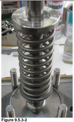
Put the bottom spring plate, the spring and the top spring plate on one after the other.
