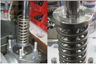
Put the spring and the upper spring disk on the lower spring disk.
