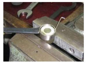
Fig. 4 Installing the snap ring
