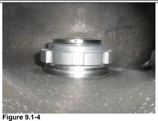
Screw the blow down ring completely down to the nozzle.
