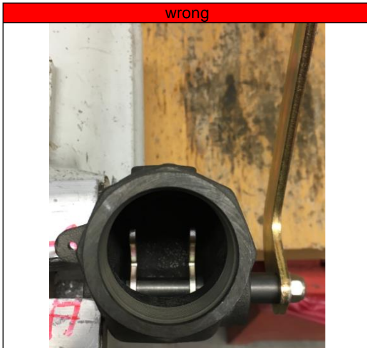
Lifting fork assembled wrong (position)
