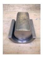
The nameplate has to be placed with its inscription upside down in longitudinal direction in the punching tool (cavity). The required form is achieved by 2-3 times manually hammering onto the plunger.
