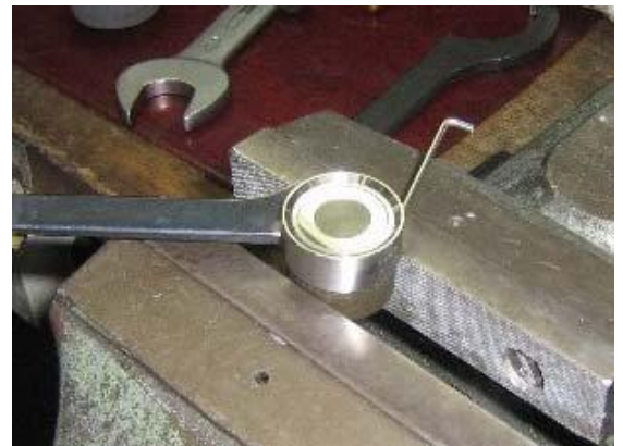
Fig. 4 Installing the snap ring
