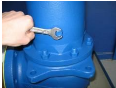
Fig. 2 Dealing the drain hole
