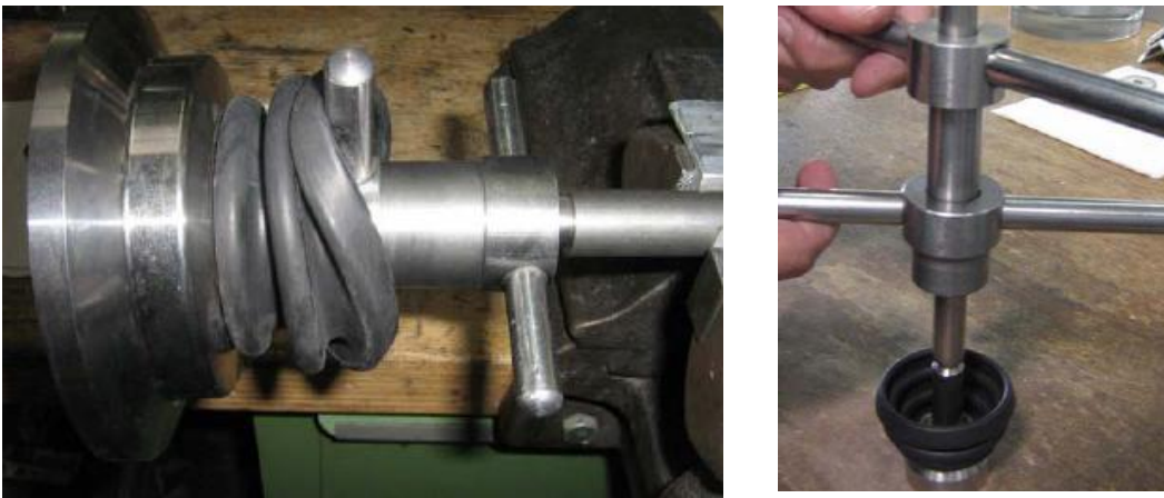
Fig. 7 Installation of the Elmoster bellows
