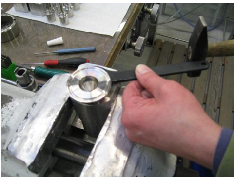
Fig. 5 Installation of the O-ring disc with a pin-type spanner wrench
