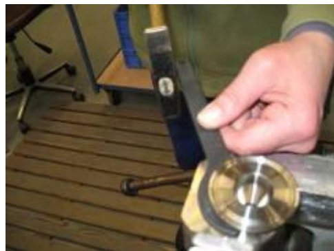
Fig. 6 Installation of the O-ring disc
