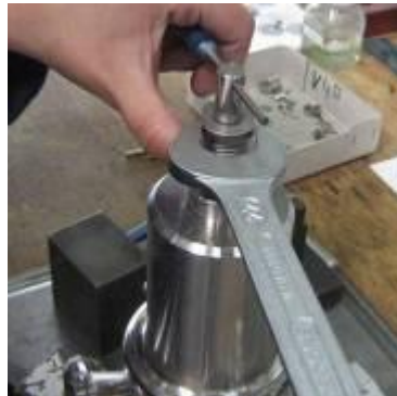
Fig. 2 Pressure setting of the safety valve
