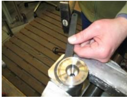
Fig. 4 Installation of the O-ring disc
